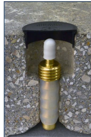
Soil vapor sample point to be used at each house.
